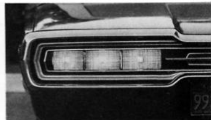
FAMOUS LIGHTS – As can be seen in this sequence of flashing tail light photos, the 1966 Thunderbird had one of the most distinctive turn signals ever devised for an automobile. This same bank of lights also doubled as brake and tail lights.
