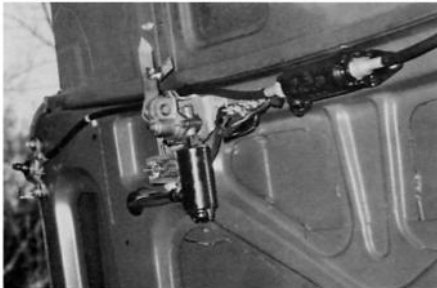
PACKAGE TRAY — The center (left) package tray motor and control switches are located here. At the far left can be seen the locking screw mechanism.
